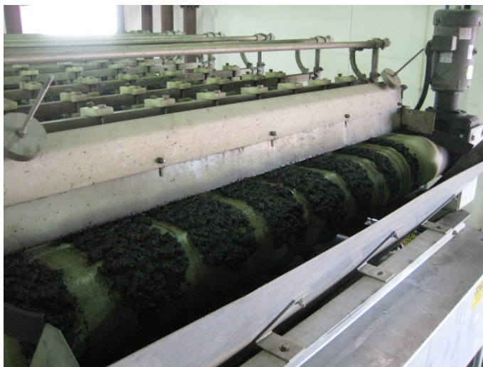
A Belt Filter Press at Hartford WPCF (Biosolids Dewatering)
